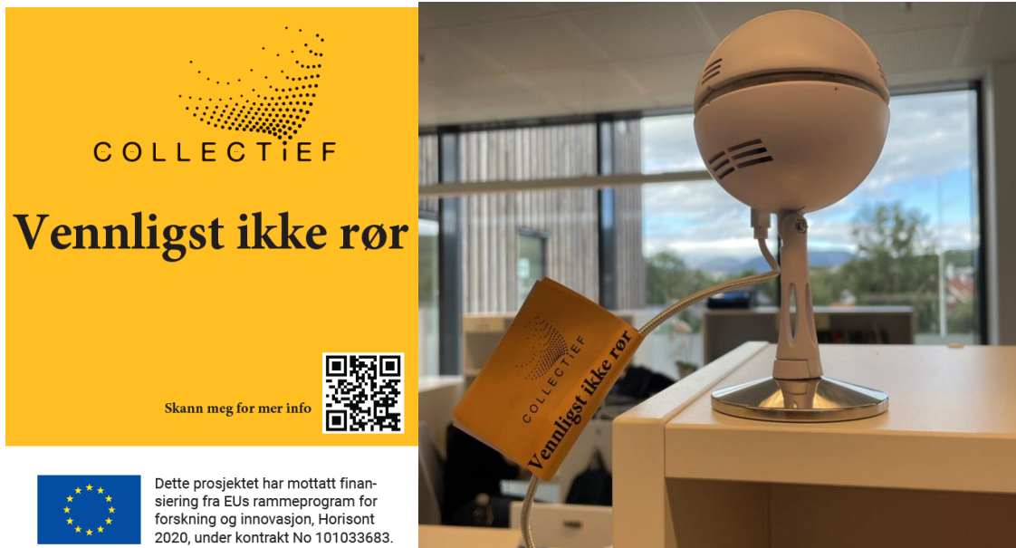
Figure 30 Installation of Sphensors in a Norwegian pilot building
